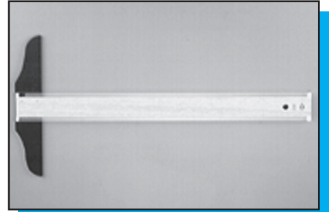
Figure 2-17 Example of a T square (Courtesy of Teledyne Post)
