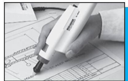
Figure 2-12 The electric eraser is the most efficient cleaner. (Courtesy of Koh-I-Noor)
