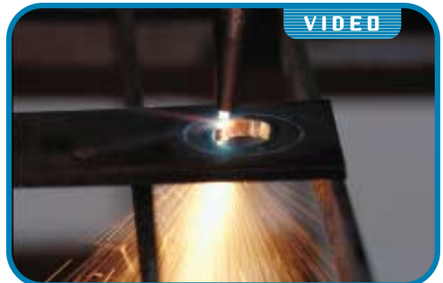
FIGURE 7-37 As a hole is cut, the center may be overheated. Courtesy of Larry Jeffus. See DFW video series.
