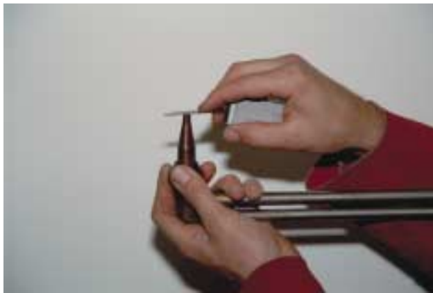
FIGURE 7-19 File the end of the tip flat. Courtesy of Larry Jeffus.
