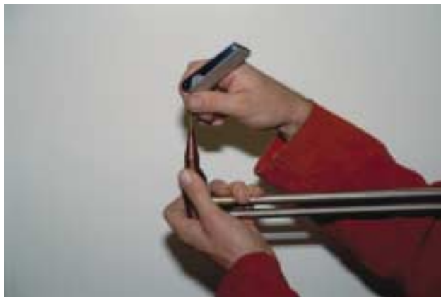
FIGURE 7-20 A tip cleaner should be used to clean the flame and center cutting holes. Courtesy of Larry Jeffus.
