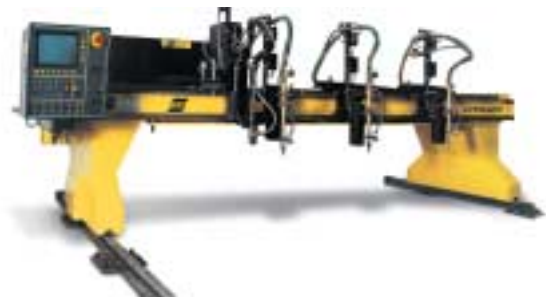
FIGURE 7-7 Multiple head cutting machine. Courtesy of ESAB Welding & Cutting Products.
