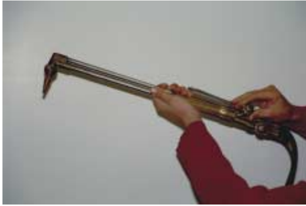
FIGURE 7-18 Turn on the oxygen valve. Courtesy of Larry Jeffus.
