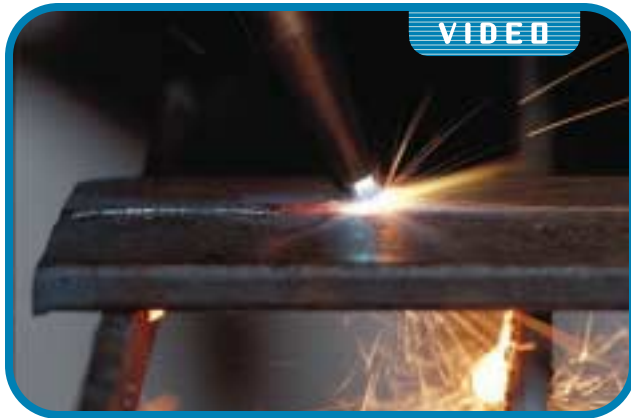
FIGURE 7-43 A good cut showing a steady stream of sparks flying out from the bottom of the cut.
