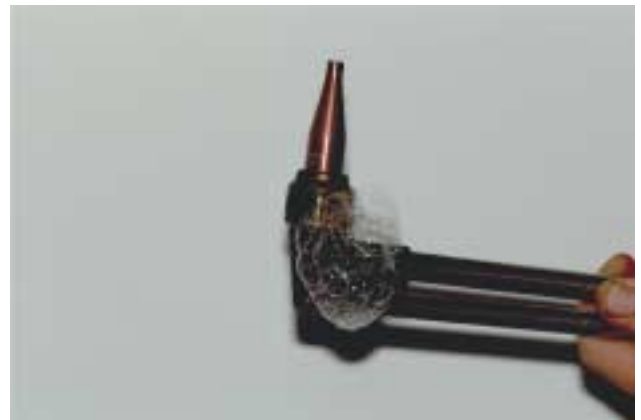
FIGURE 7-15 Checking a cutting tip for leaks. Courtesy of Larry Jeffus.
