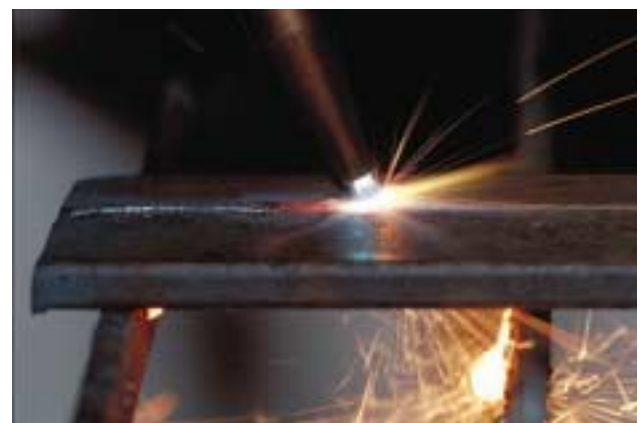
FIGURE 7-58 The torch is rotated to allow the preheating of the plate ahead of the cut. This speeds the cutting and provides better visibility of the line being cut. Courtesy of Larry Jeffus.
