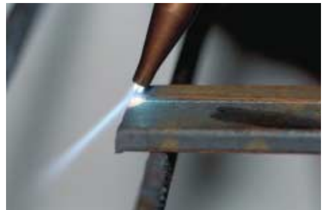
FIGURE 7-57 Beginning a cut with the torch concentrating the flame on the thin edge to speed starting.
