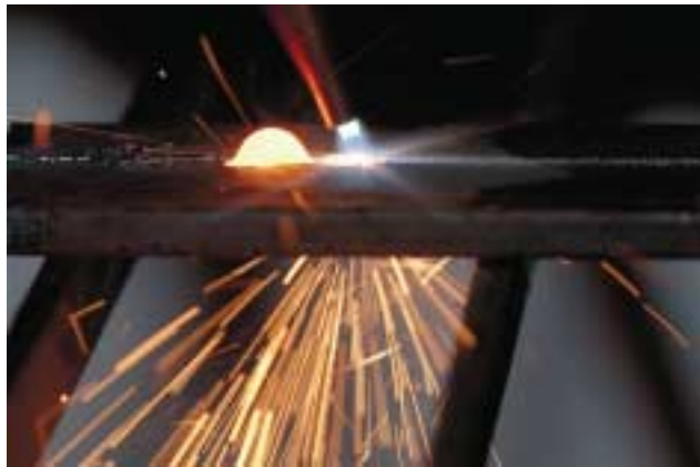
FIGURE 7-44 Poor cut. The slag is backing up because the cut is not going through the plate. Courtesy of Larry Jeffus.
