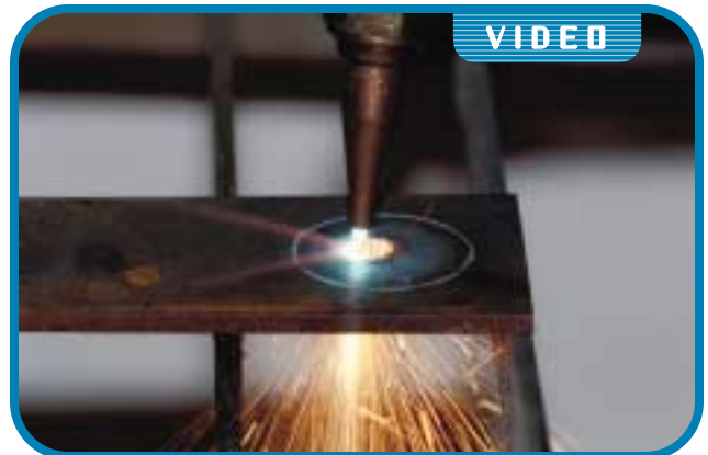
FIGURE 7-36 The sparks from cutting a mild steel plate, 3/8 in. (10 mm) thick, 6 ft (1.8 m) from the floor, will be thrown much farther if the cutting pressure is too high for the plate thickness. These cuts were made with a Victor cutting tip no. 0-1-101 using 25 psig (1.7 kg/mm 2 ) as recommended by the manufacturer and by excessive pressures of 45 psig (3.1 kg/mm 2 ) and 65 psig (4.5 kg/mm 2 ).
