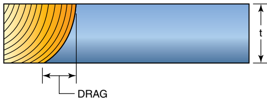
FIGURE 7-30 Drag is the distance by which the bottom of a cut lags behind the top.
